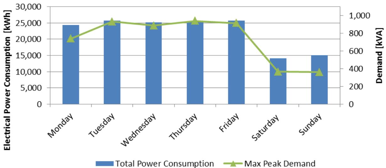
Figure 3 Weekly electricity consumption profile at a non-rendering site Category D (AMPC DPEEP, 2012)
