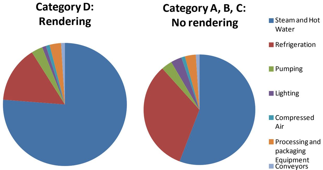
Figure 7: Energy consumption by equipment.
