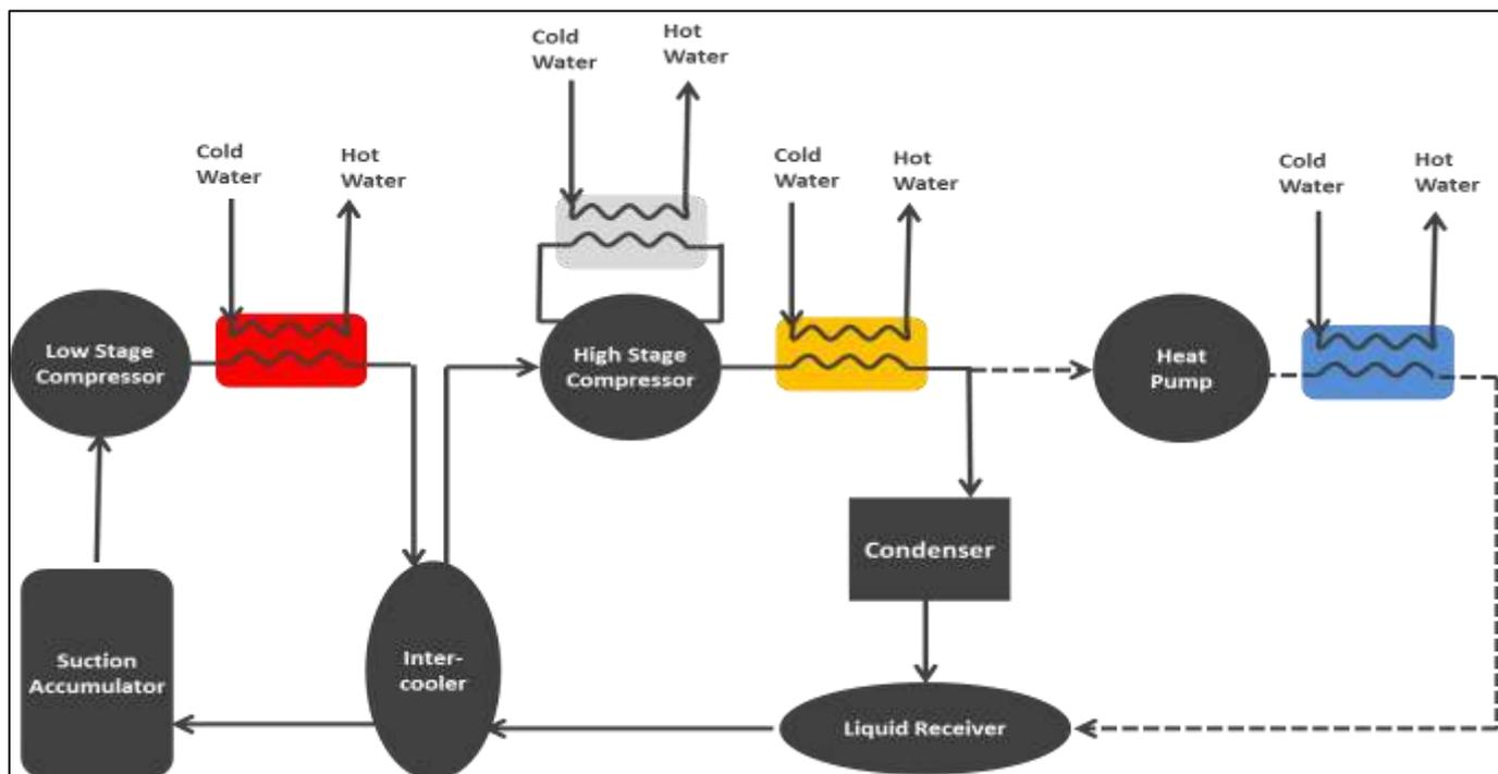
Figure 2 – Schematic depicting the main heat recovery options shown in Table 1.
