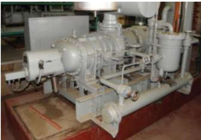
Figure 1 - Old Stal screw compressor package.
