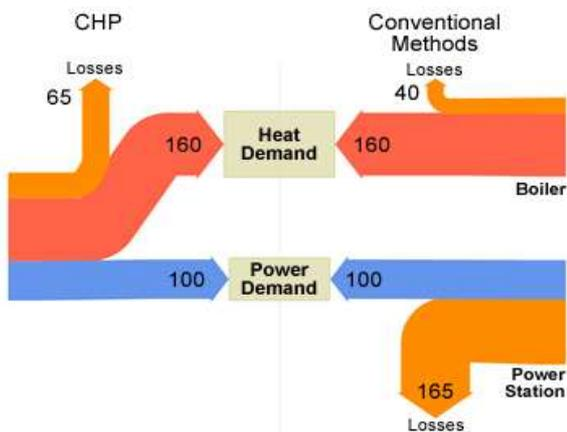
Figure 1 Energy flow diagram comparing conventional methods and cogeneration (CHP)<sup>2</sup>
